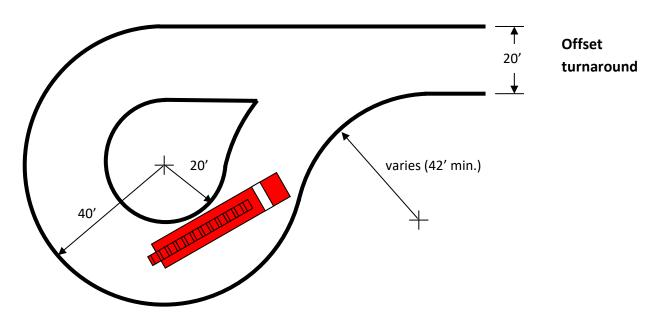
NOTE: Parking is not permitted in any of these hammerheads at the dimensions shown.
