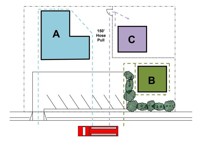
Assume that the parking lot is not accessible to fire apparatus due to turning radii and fire lane widths less than the required minimums.
