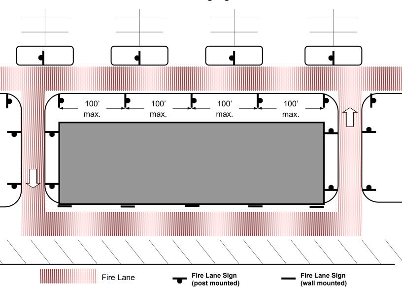
Signs are required within 3' of the end of each designated fire lane and spaced a maximum of 100' along the entire designated lane. One sign is required for each island adjacent to the fire lane.
