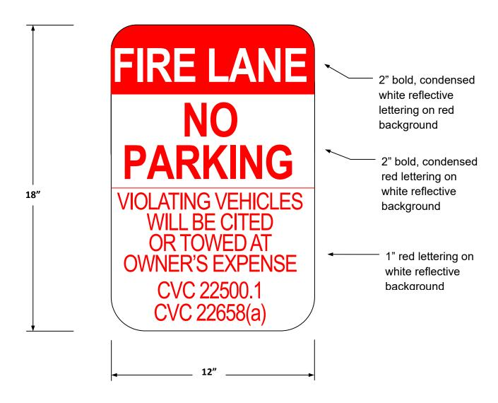
All sign and lettering dimensions shown are *minimums*. "Arial Narrow" font used in sample above, though other legible sans-serif fonts may be acceptable.
